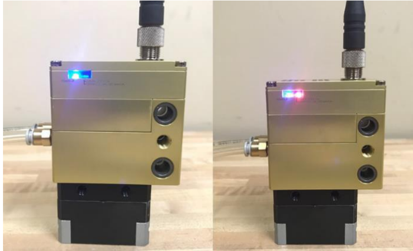
Figure 4: Magswitch J30 Startup Sequence – Power LED 1 (blue) and Magnet LED 2 (red) illuminated when complete
